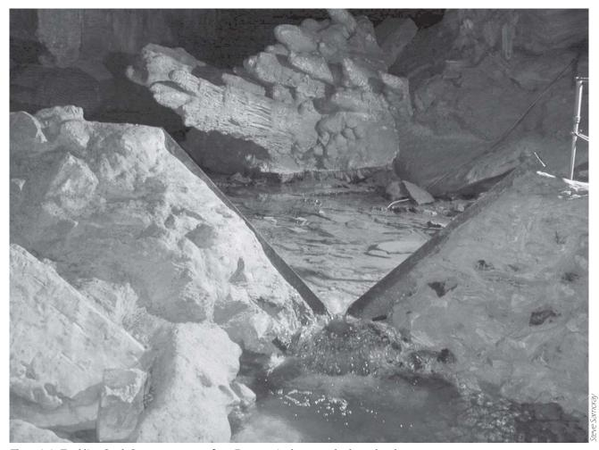
The weir in Tumbling Creek Cave gauges water flow. Detectors in the stream lead to a data logger.
